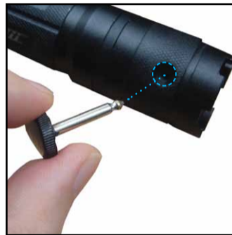
Removing the Safety Interlock from the Encap will disable the laser.
